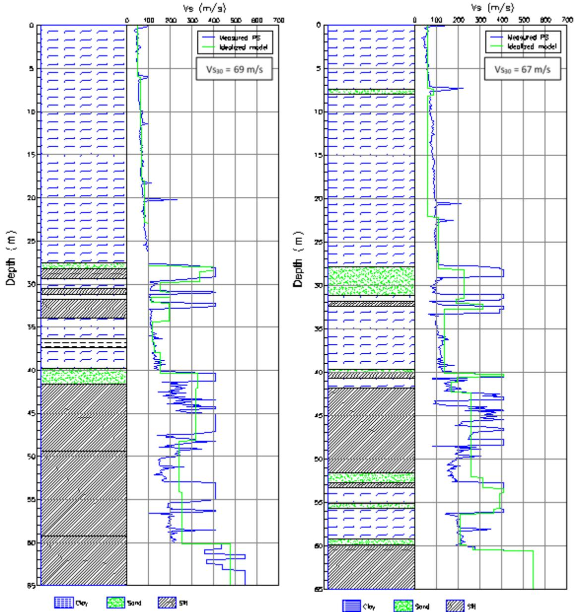
Figure 5. Typical soil profiles for Zone III (Mayoral et al., 2016)
