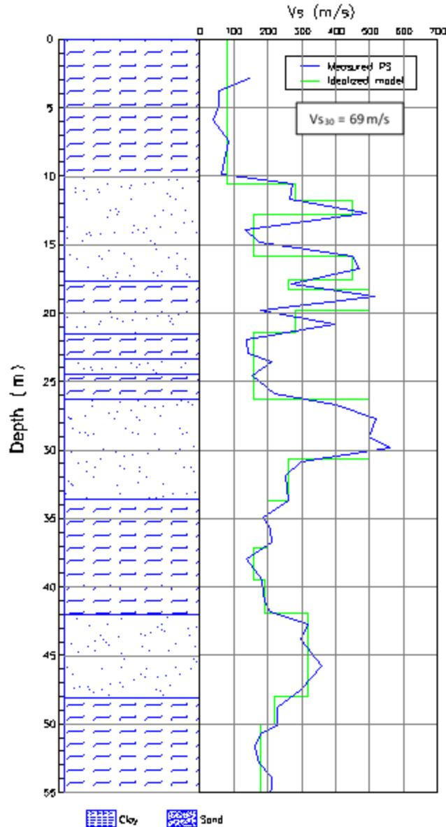
**Figure 7.** Typical soil profile for the Transition Zone (after Mayoral et al., 2016)
