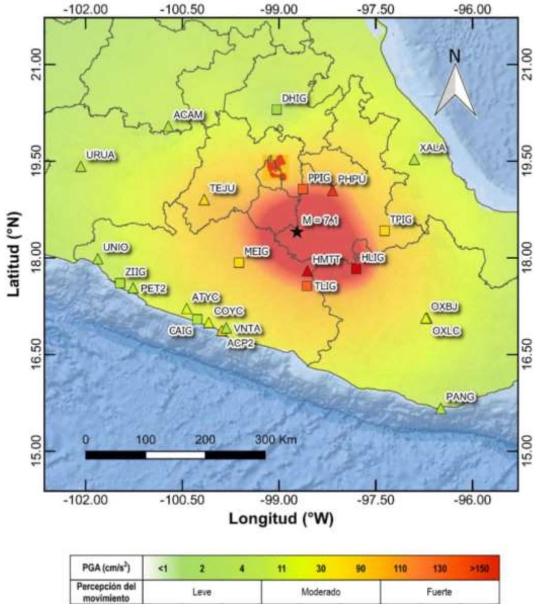
Figure 14. Regional PGA (cm/sec<sup>2</sup>) map from the September 19 Mw 7.1 event (after IINGEN 2017)
